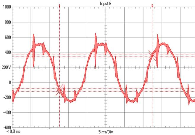
Fig. 11. Voltage waveform at input to harmonic filter.
