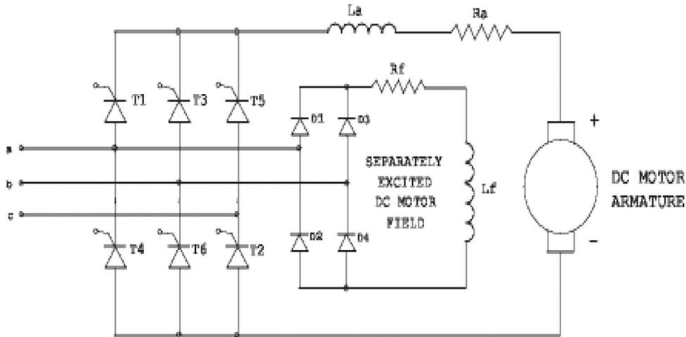
Fig. 3. Typical dc drive and motor schematic.
