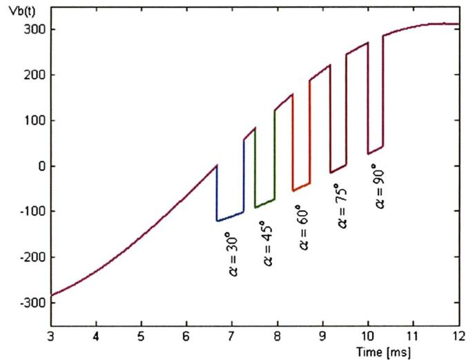
Fig. 6. Notch-depth variations on firing-angle changes [4].
