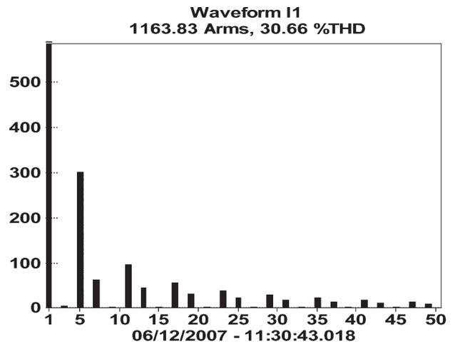
Fig. 14. Harmonic current spectrum of 700-hp dc press drive before treatment.  $I_{thd} = 30\%$ .
