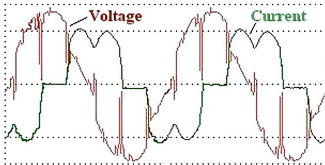
Fig. 4. Commutation notches on voltage supply due to fully controlled SCRs on dc drilling drives [3].
