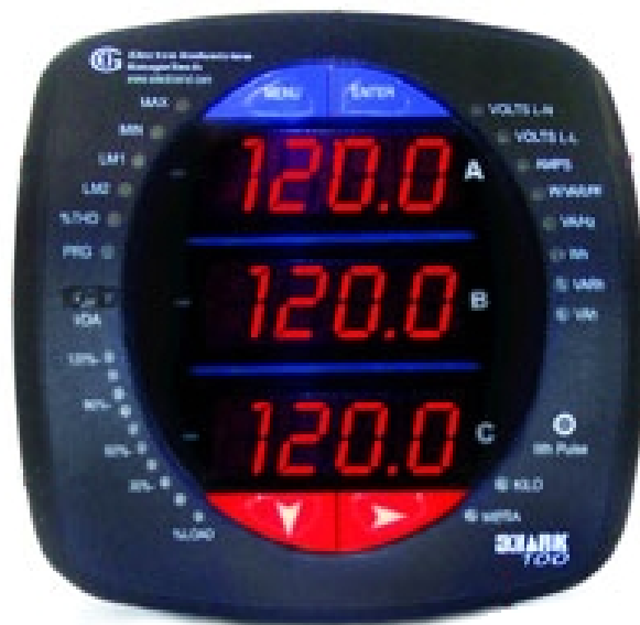
Figure 1-5 Power Monitor Front Panel
