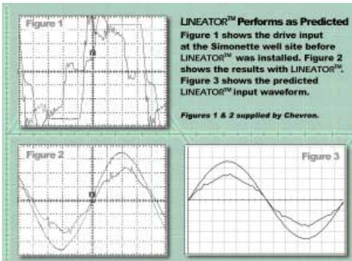
Engineers at Chevron decided to take preventive measures to limit harmonics at well sites. For applications where a low voltage drive is the only non-linear load, and when it is a relatively low horsepower (1000 HP or less), Chevron selected Mirus' LINEATOR™ Universal Harmonic Filter (UHF).
